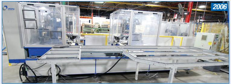
STURTZ CNC-2K-30-F 2-HEAD CORNER CLEANER, 16-1/2" MIN, 120"W MAX, 1" – 6" PROFILE HEIGHT, SELF-CLEANING BELT SYSTEM, PC MONITOR SYSTEM, MOVABLE HEAD POSITIONING BAR CODE SCANNER, S/N 40109
