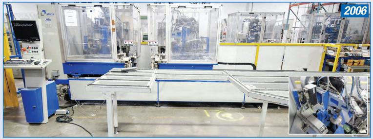
STURTZ CNC-2K-30-F 2-HEAD CORNER CLEANER, 16-1/2" MIN, 120"W MAX, 1" -6" PROFILE HEIGHT, SELF-CLEANING BELT SYSTEM, PC MONITOR SYSTEM, MOVABLE HEAD POSITIONING BAR CODE SCANNER, S/N 40094
