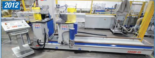
**STURTZ** SD500 AUTOMATIC DUAL MITRE SAW, AUTO ANGLE ADJUSTMENT (90-45 DEGREE) W/ SELECTOR SWITCH, INDEPENDENT HEAD OPERATION, S/N 28957
