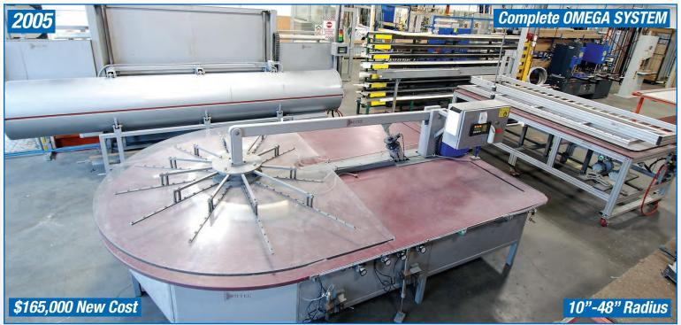
SYN-TEC DRY VINYL BENDING SYSTEM WITH OMEGA 2000 RADIUS TABLE WITH HIGH THROUGHPUT EXTREME PRECISION UNIVERSAL TOOLSET FOR RADII FROM 10" TO 48", ELECTRIC DRIVE. SMOOTH 8' X 12' TABLE SURFACE FOR CONTINUOUS JAMBS, PNEUMATIC CLAMPING & ELECTRIC OVERPRESS S/N S-025, OMEGA 6000 RADIANT HEAT WITH 8 ELEMENTS, TWO ZONE CONTROL, MULTIPLE PROFILES OF ANY LENGTH, 14' HEATING ZONE, CIRCULAR DESIGN FOR EVEN HEAT PENETRATION, S/N HC-016, OMEGA SEGMANT TABLE
