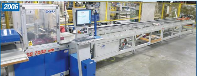
STURTZ SD7000 AUTOMATIC CNC SAW, 18" X 25' INFEED TABLE, 2 PLC CONTROL PUSH BAR, 6 CLAMPING CYLINDER, S/N 21133
