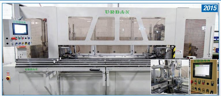
URBAN SV 350 2-HEAD CORNER CLEANER, 2-HEAD X 2-AXIS TOOL MOVEMENT, INSIDE/OUTSIDE CLEANING, (7) STANDARD TOOL POSITIONS PER HEAD, DISC CUTTER, 210MM – 2,200MM FRAME WIDTH, 20MM – 300MM PROFILE HEIGHT, S/N C41037
