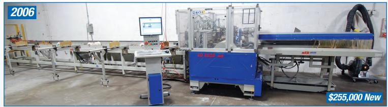
STURTZ SD8000 CNC DUAL MITRE SAW, S/N 21538, 21'L, 6" MIN CUT, NOTCHING 1-12 DEGREE, 18" X 25' INFEED TABLE, PLC CONTROL, (17) FABRICATION TOOLS ON 3-AXIS, 6-CLAMP, S/N 21538
