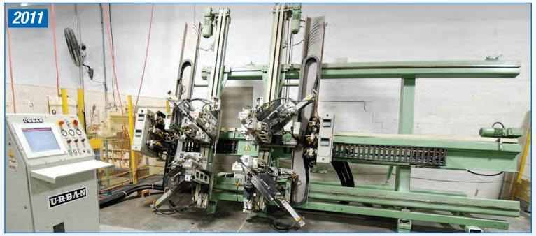
URBAN AKS 1900 37/22 4-POINT CORNER WELDER, 146" X 87" MAX DIMENSIONS, 50MM - 200MM PROFILE HEIGHT, S/N C07030
